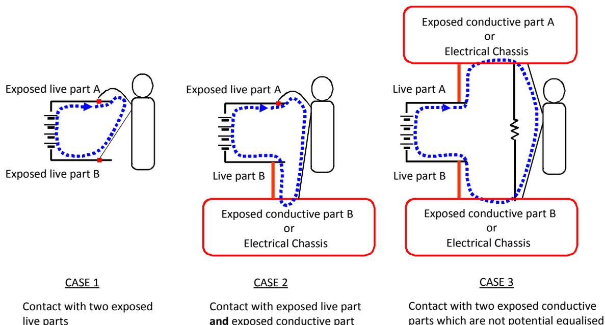
**Figure 1: Possible electric shock path cases**
