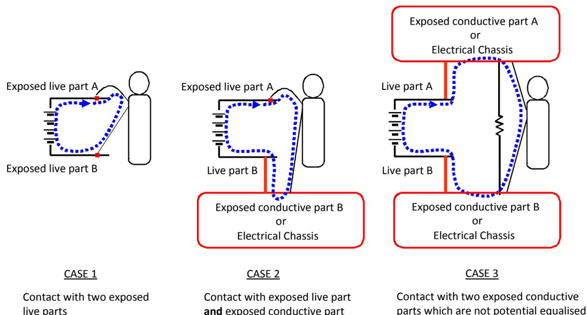
**Figure 1: Possible electric shock path cases**
