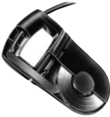
The Magne-Charge plastic 'paddle' is seen here in cutaway showing the magnetic induction coils.
