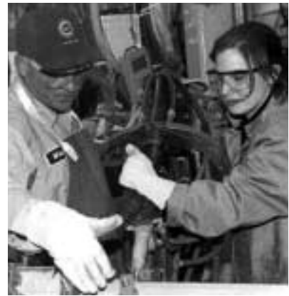
Craftsman skills are needed to apply the continuous strip of structural adhesive.
