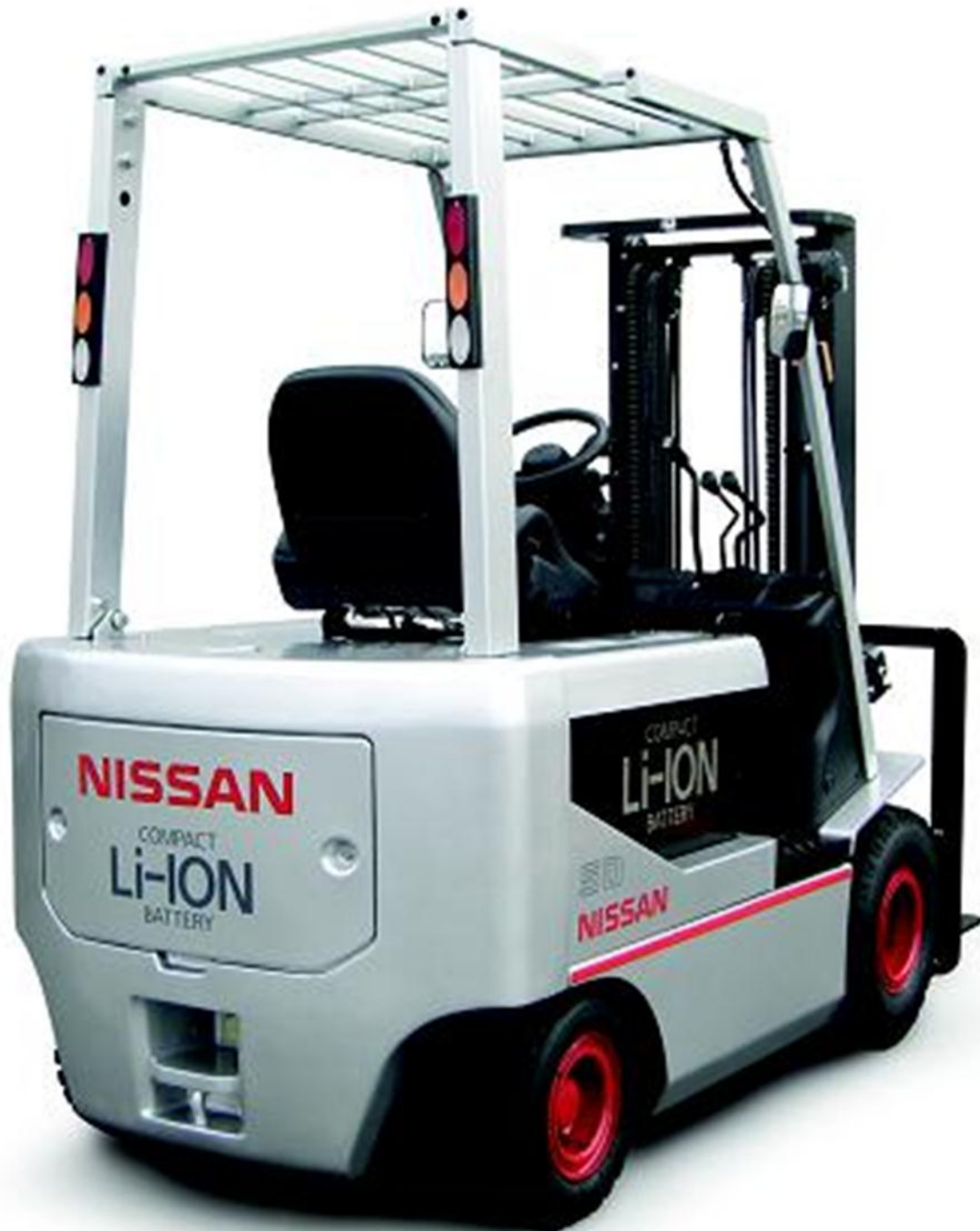
Fig. 2.6 Pure electric forklift truck with the new lithium-ion battery improving performance and reducing down time and labour costs
