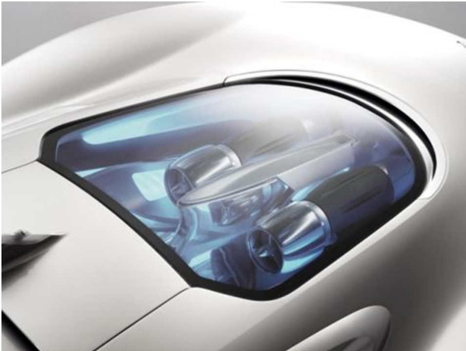
Fig. 3.1 Planned Jaguar supercar with two micro turbine range extenders generating 140kW total
