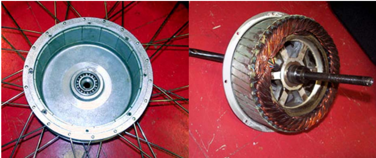
Fig. 1.5 Bicycle hub motor rotor left and stator right.
