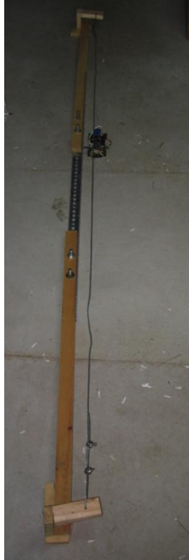
Figure 2. The stationary recharging system. The 3 m stainless steel cable is suspended approximately 10 cm above the floor. The RC car can be seen traveling under the system.
