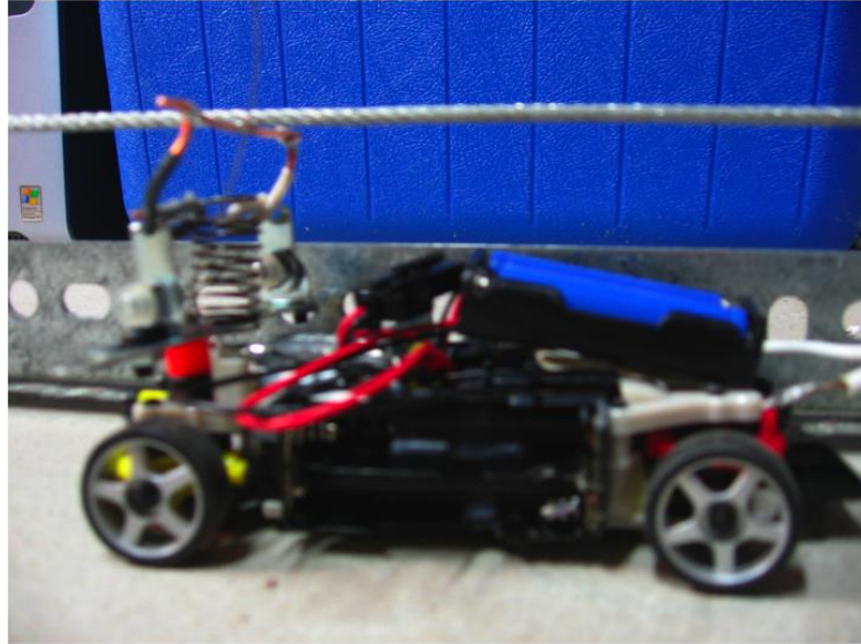
Figure 3. The RC car with the prototype pantograph system installed. The top of the pantograph is touching the stainless-steel wire that supplies electricity to the system.
