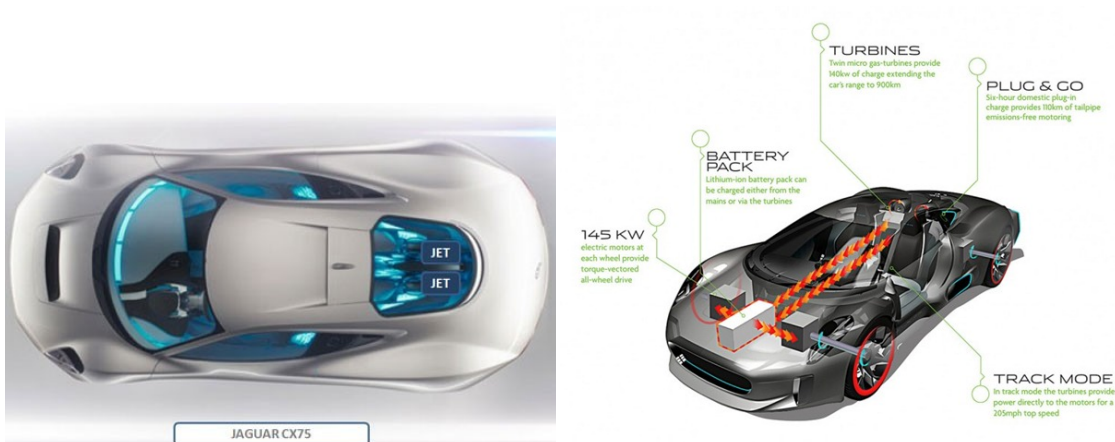
Fig. 1.5 Jaguar CX75 supercar with jet turbine range extenders
