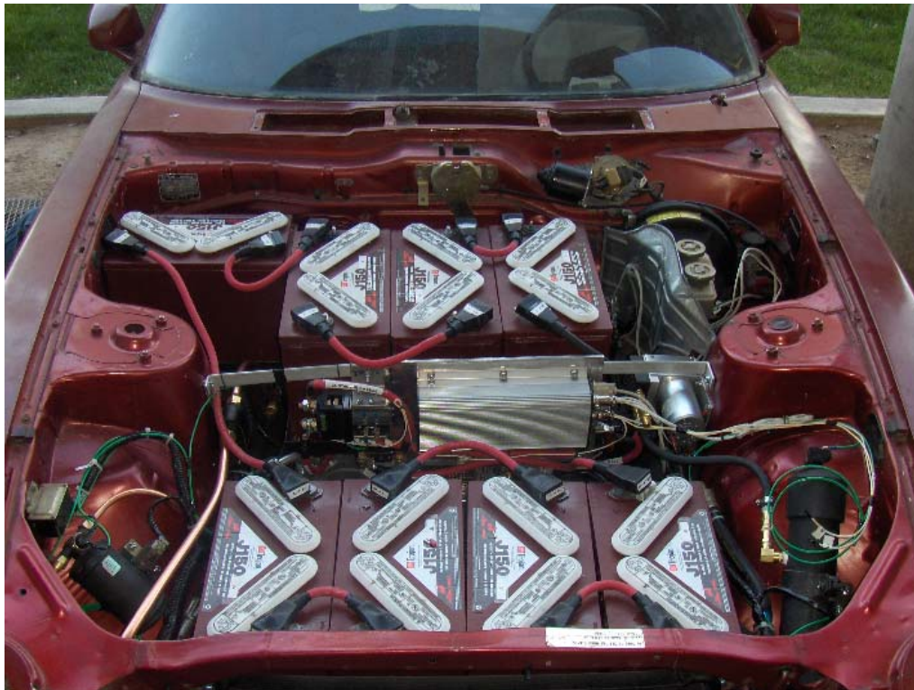
Figure 4: Batteries and motor controller mounted under the hood.
