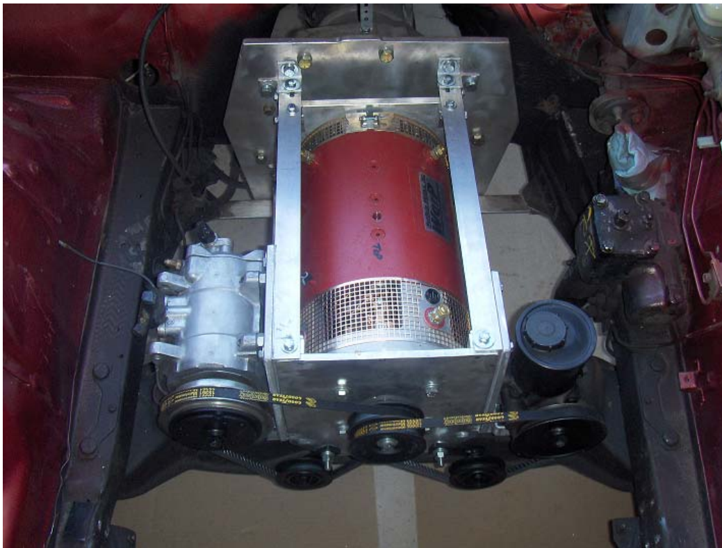
Figure 3: Motor mounted with power steering (right) and air conditioning compressor (left)
